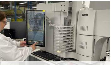
The LECO Combustion IR can report levels of sulfur down to 0.01% or 100 mg/kg
